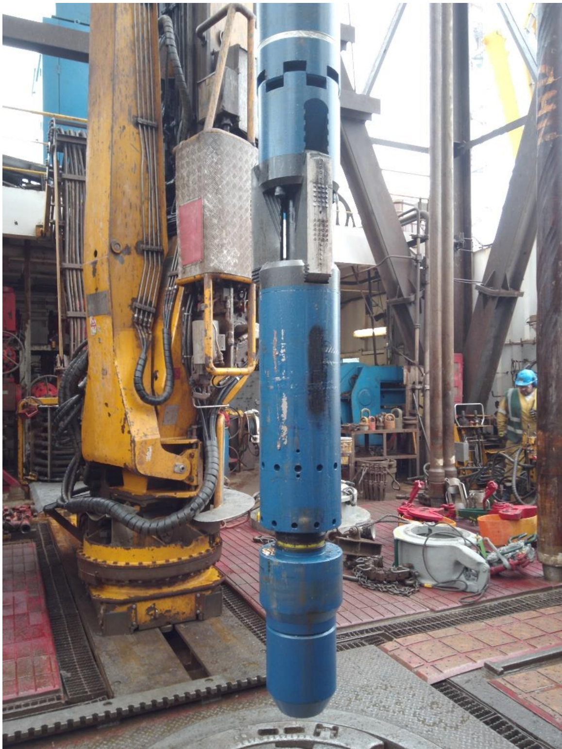
Figure 1: Drill-pipe deployed anchor
